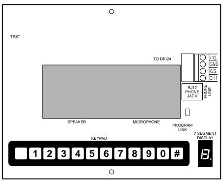
Figure 1: The DT1 with its outer cover removed.
